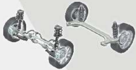
MacPherson Strut front and Torsion Beam rear suspensions for a smooth and pleasurable drive.
